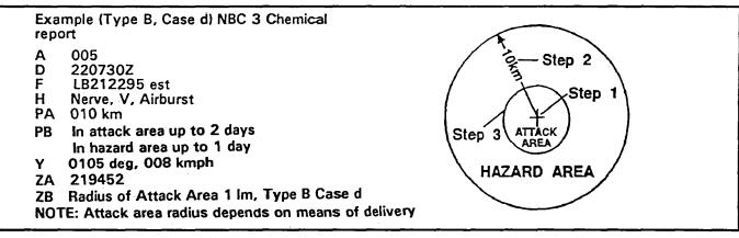
Figure 3-18. Plot for downwind hazard, Type B, Case d.
